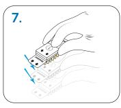
Tap firmly 2-3 times, repeating if air-bubbles are visible in the wells
