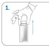
Put on clean gloves and remove a twin (HiSCC) cartridge from packaging
