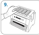
Insert cartridge into Lapbox with the arrows facing to the back, and replace the lid
