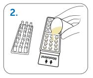
Remove cartridge lid and place upside down. Half-fill chamber 1 with milk sample 1.
